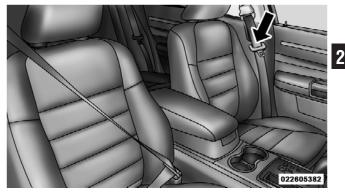
Pulling Out the Lap/Shoulder Belt Latch Plate
